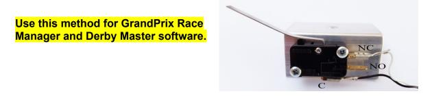
If you want the switch to be un-pressed before the race and pressed when the race starts, then the push-on terminal needs to be on the NO contact as indicated below.
